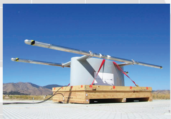
Left: Aerodynamic North Atlantic Treaty Organization (NATO) mount supports twin broadband Very High Frequency dipoles. Right: Close-up view showing the attachment of the antennas and mount on the C-131 aircraft.
