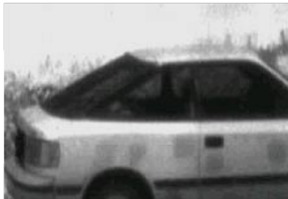
Imaging picture taken by a 320x256, 9.7 \mu\text{m} , heterojunction, LWIR HgCdTe camera showing repair areas.
