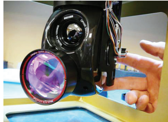
Figure 1 (left): Close-up picture of the Aerius Compact Laser Illuminator (CLI) module. The illuminator uses a small Aerius Vertical-Cavity Surface Emitting Laser (VCSEL) chip that produces narrow-band illumination in the short-wavelength infrared (SWIR) band. Figure 2 (right): Aerius illuminator mounted and bore sighted with the customer's system.
