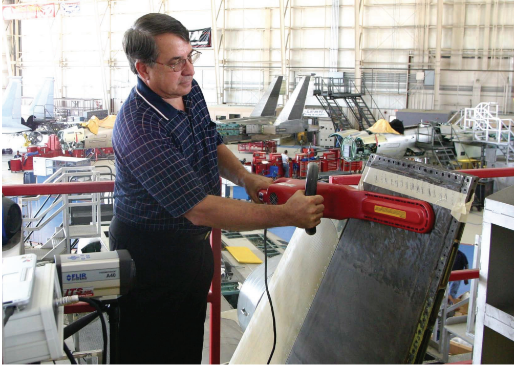
Induction Thermography System Inspection at Robins AFB, Georgia
