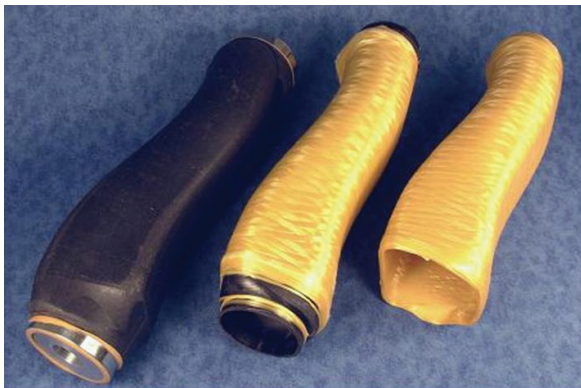
Shape memory polymer-based tooling offers benefits in materials and labor costs (Photo: CRG SMP copyright 2007)
