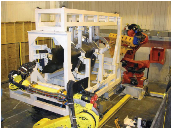
Left: An Inlet Duct Robotic Drilling (IDRD) cell at work. Right: An artist's concept of IDRD cells.
