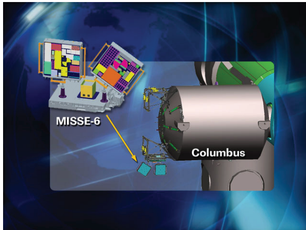
Left: Graphic showing location of the Materials on the International Space Station Experiment-6 (MISSE-6) experiments on the exterior of the International Space Station. Right: MISSE-6 tray that includes ATEC's heat-flux based emissivity (HFBE) module after all the experiments were attached.
