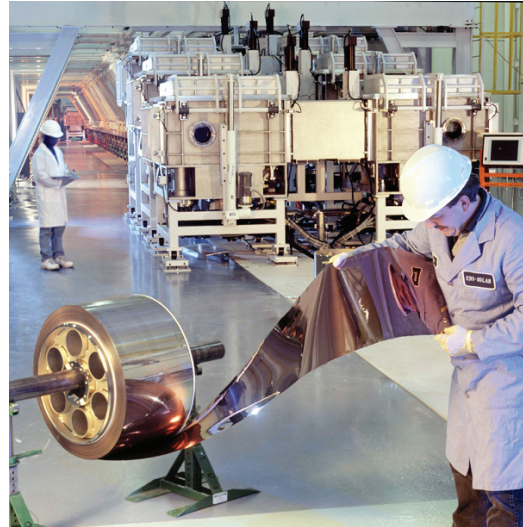
Left: United Solar Ovonic thin-film photovoltaic (PV) material is flexible, durable, and lightweight. Right: UNI-SOLAR® PV material being produced.
